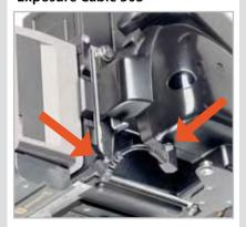
Hasselblad 503CW plus Winder CW with Exposure cable 503 in place showing connection from Winder to adapter.
